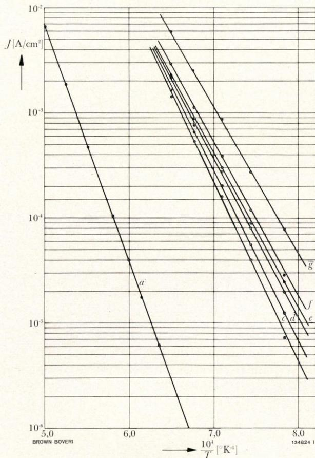
Fig. 1. - Richardson lines for tantalum coated with thorium or thorium oxide
