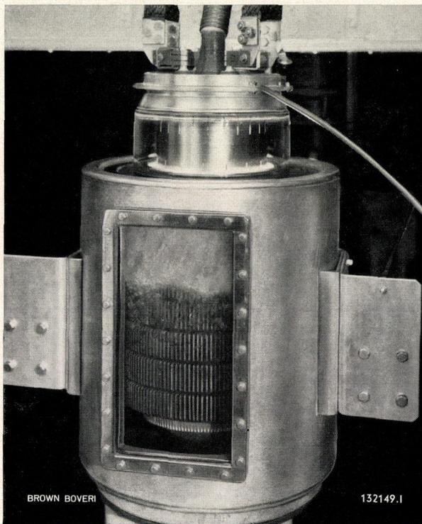
Fig. 6. - The BTS 150-2 in its boiler on the test stand
