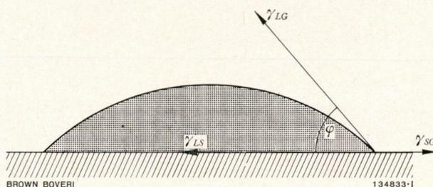
Fig. 1. — Surface tensions of a liquid droplet at the liquid-solid  $\gamma_{LS}$ , liquid-gaseous  $\gamma_{LG}$ , and solid-gaseous  $\gamma_{SG}$  interfaces on a solid surface with contact angle  $\varphi$
