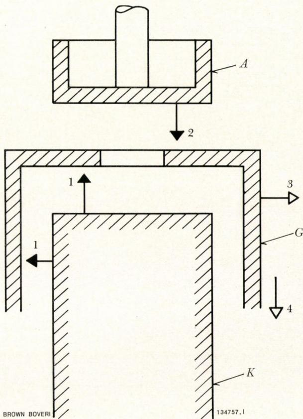
Fig. 2. - Heat balance of a thyatron grid
