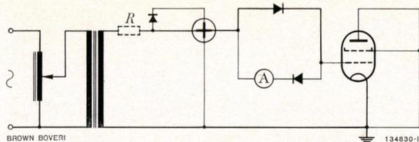
Fig. 5. - Basic circuit diagram of apparatus for measuring  $I_{gp}$
