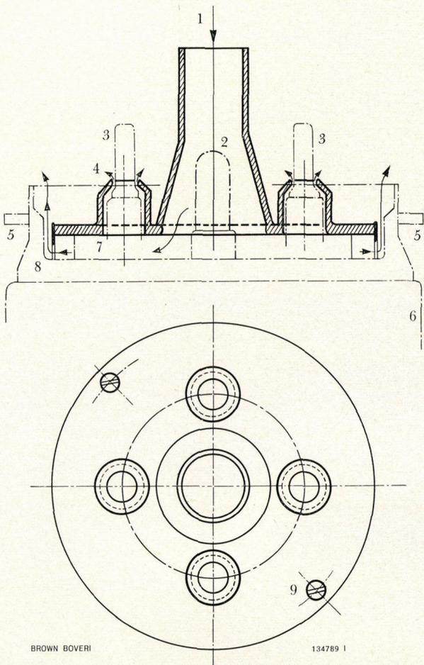
Fig. 4. - Cooling-air supply to the base
