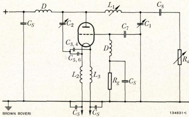
Fig. 8. - Basic circuit diagram of the test oscillator
