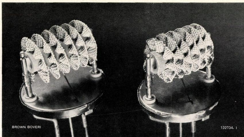
Fig. 7. — Right, an oxide-coated cathode damaged by repeated short circuits, left, an undamaged cathode
