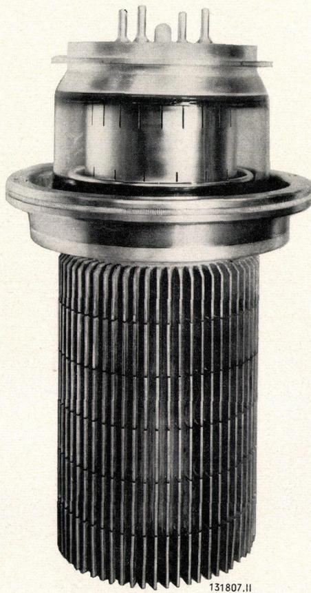
Fig. 5. - The BTS 150-2 with vapour-cooled anode
