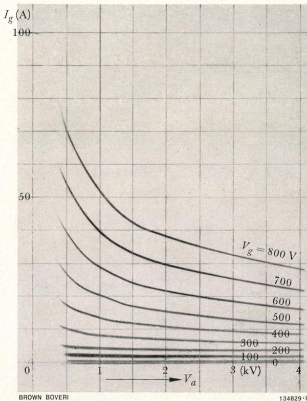
Fig. 3. - Oscillogram of characteristics  $I_a = f(V_a, V_g)$  of a high-power transmitting tube, obtained with the characteristic recorder
