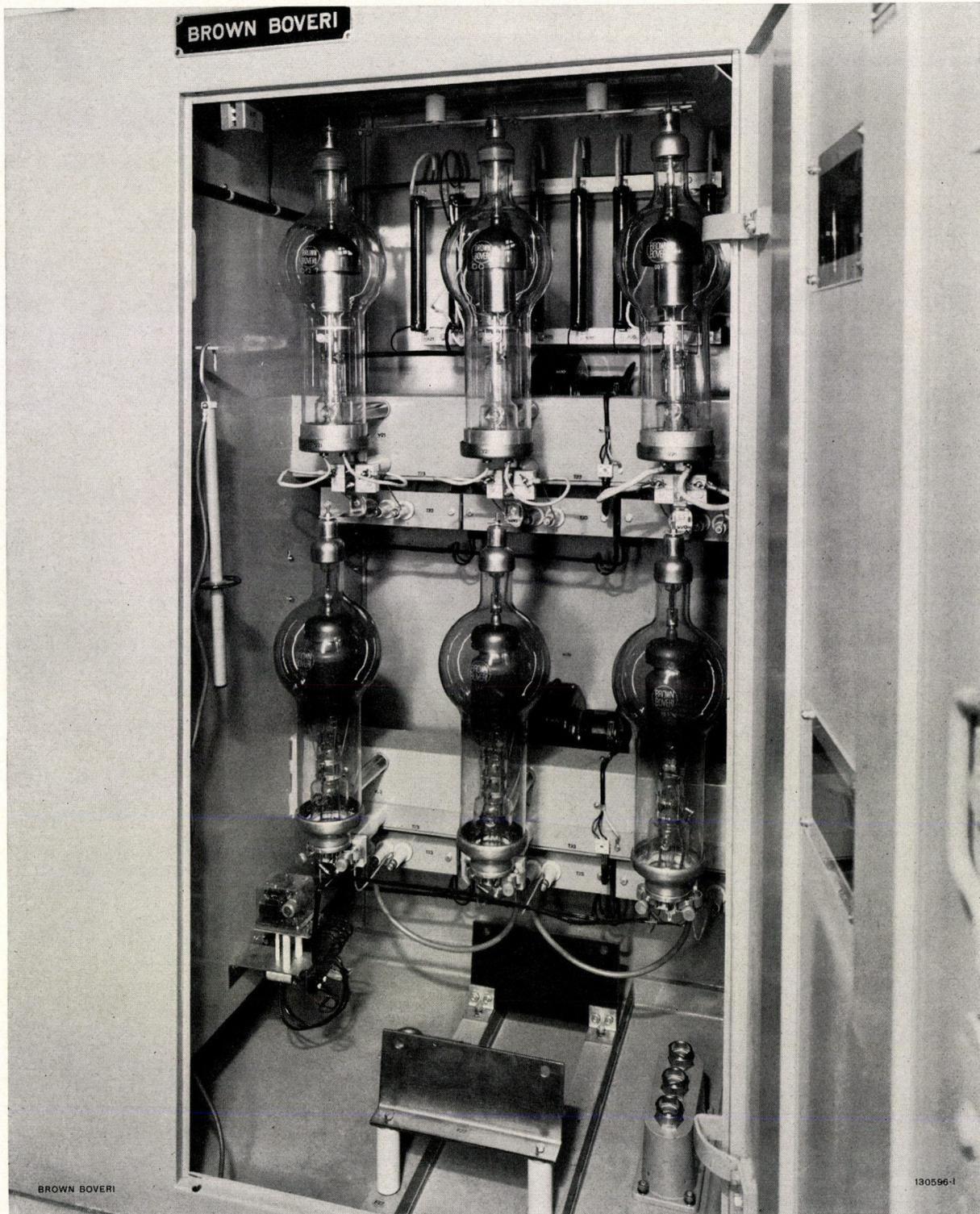
*Rectifier tubes in a high-frequency industrial generator for induction heating*
