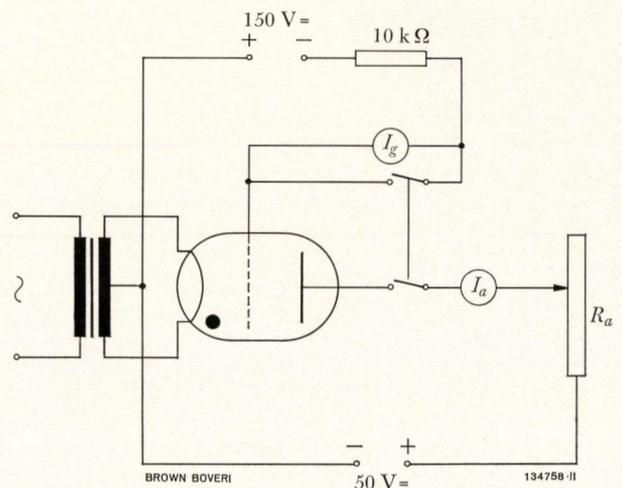
Fig. 3. – Basic circuit for measuring grid emission
