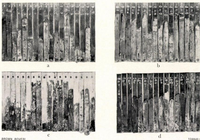
Fig. 5. — Rise heights of diverse types of soft solder on copper with various surface treatments
