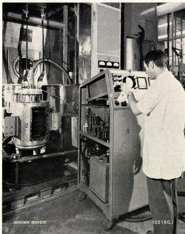
Fig. 6. - Measuring the emission of a BTS 150-2 high-power transmitting tube mounted on its test stand
