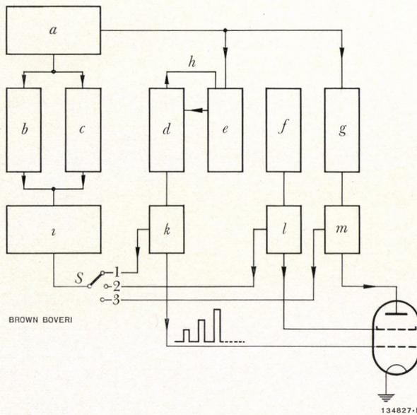
Fig. 2. — Block diagram of the characteristic recorder
