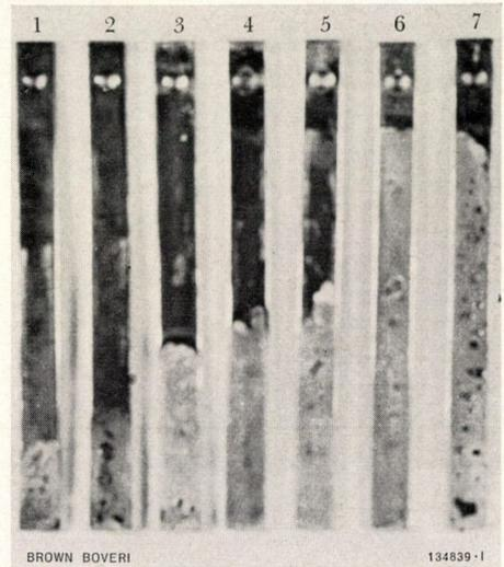
Fig. 4. — Rise heights of a tin-silver solder in a capillary gap between two copper plates using various fluxes
