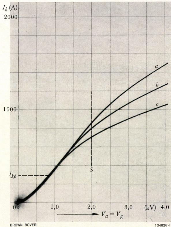
Fig. 1. - Oscillogram of the diode characteristic of a transmitting tube
