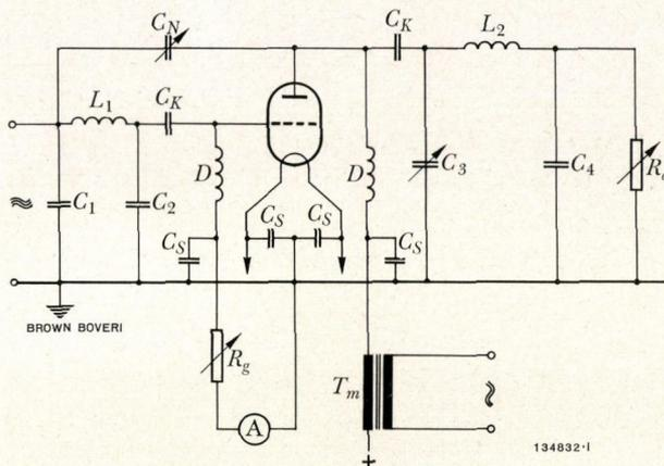
Fig. 9. - Basic circuit diagram of the anode-modulated transmitting amplifier
