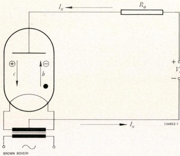
Fig. 1. - Directions taken by the electrons and ions in an ignited gaseous-discharge tube
