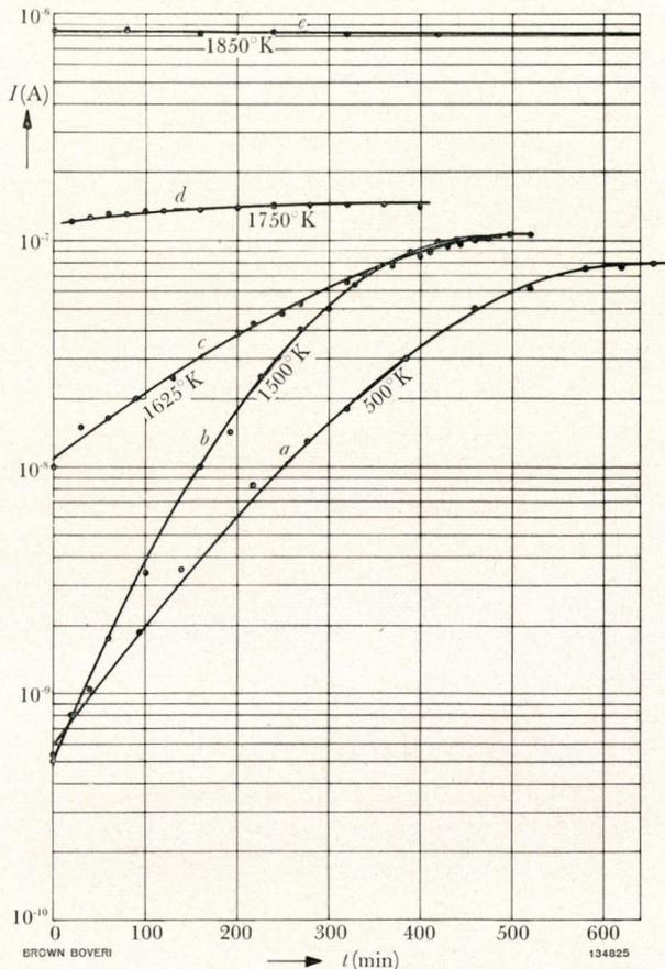
Fig. 2. - Activation of platinum coated at different temperatures with thorium
