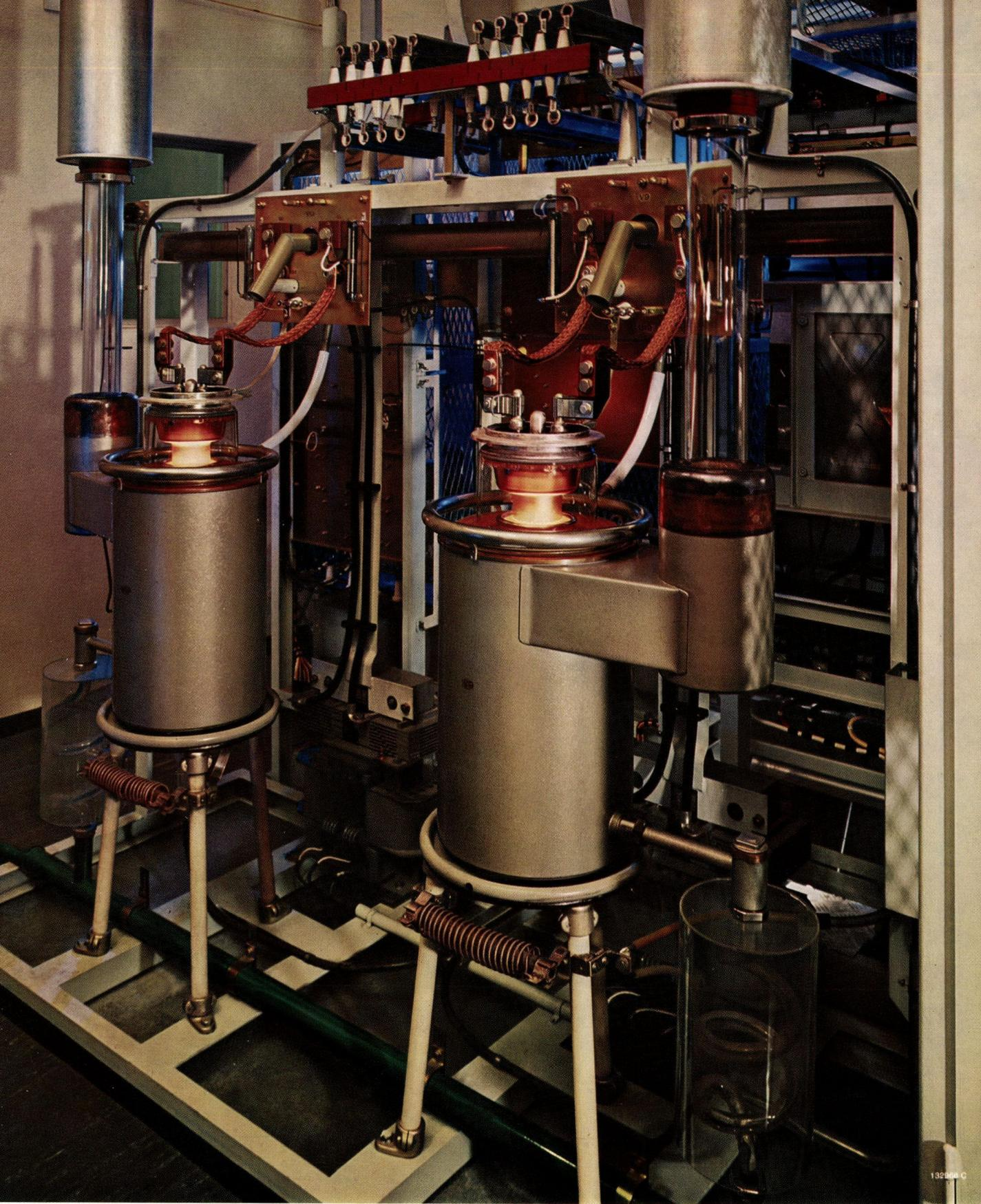
*Modulator of the 250-kW medium-wave transmitter of the Swiss national broadcasting station in Beromünster*
