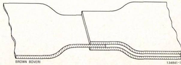
Fig. 6. - Test specimen for determining the shear strength of soldered joints
