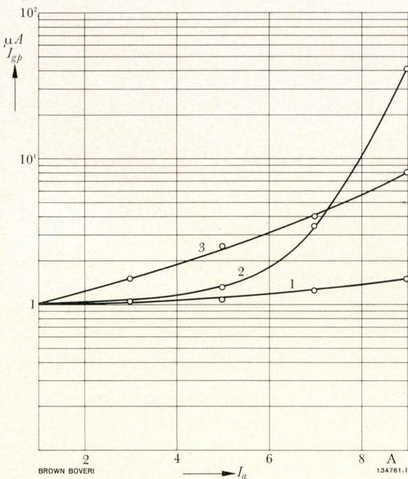
Fig. 6. - Thermal grid emission  $I_{gp}$  in relation to anode loading  $I_a$
