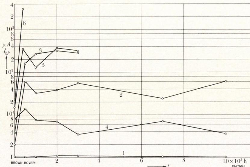
Fig. 5. - Thermal grid emission  $I_{gp}$  during life  $t$  for different grid coatings and cathode materials
