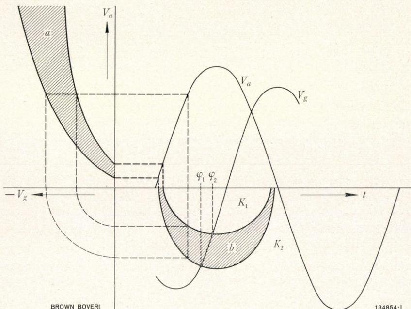
Fig. 2. - Derivation of the ignition characteristic from the control characteristic, with account taken of deviations
