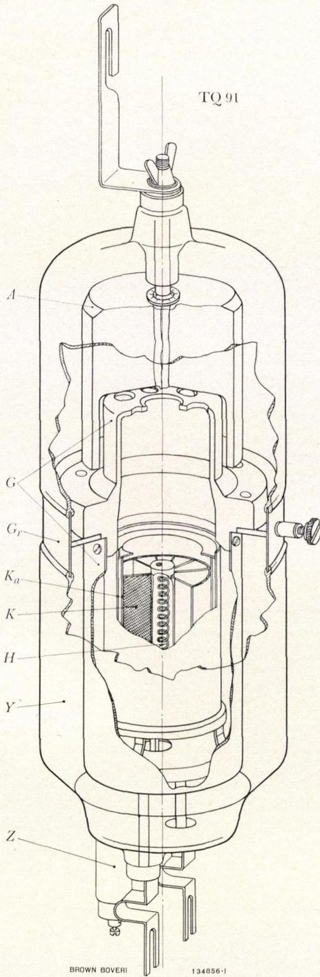
Fig. 4. - TQ 91 high-power thyatron with mercury-vapour filling
