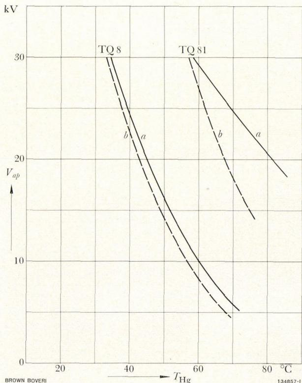
Fig. 6. — Inverse voltage characteristics of tubes TQ 8 (super-seeded) and TQ 81 (new)
