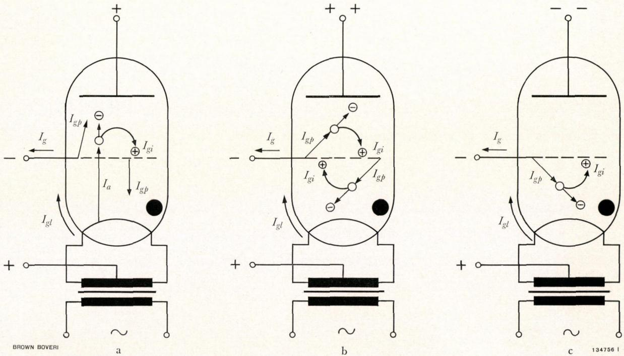
Fig. 1. — Diagrams showing the components of grid current at different stages of operation
